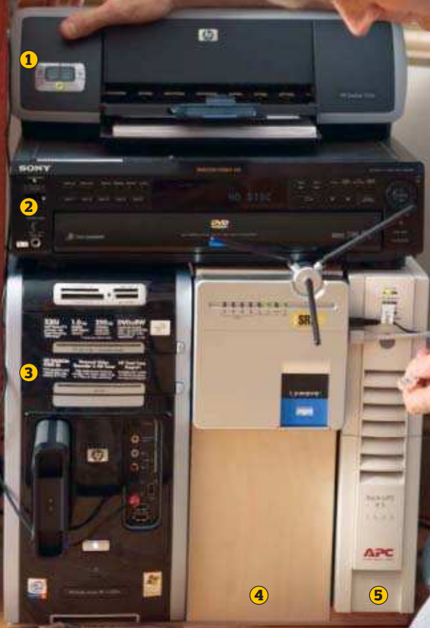
To save room, Jones stacked the hardware in his new home office. 1) HP Deskjet 5740 • 2) Sony CD-DVD Player (not provided by PM) • 3) HP Media Center PC 4) Linksys Wireless-G broadband router • 5) APC Back-UPS RS1500VA surge protector
